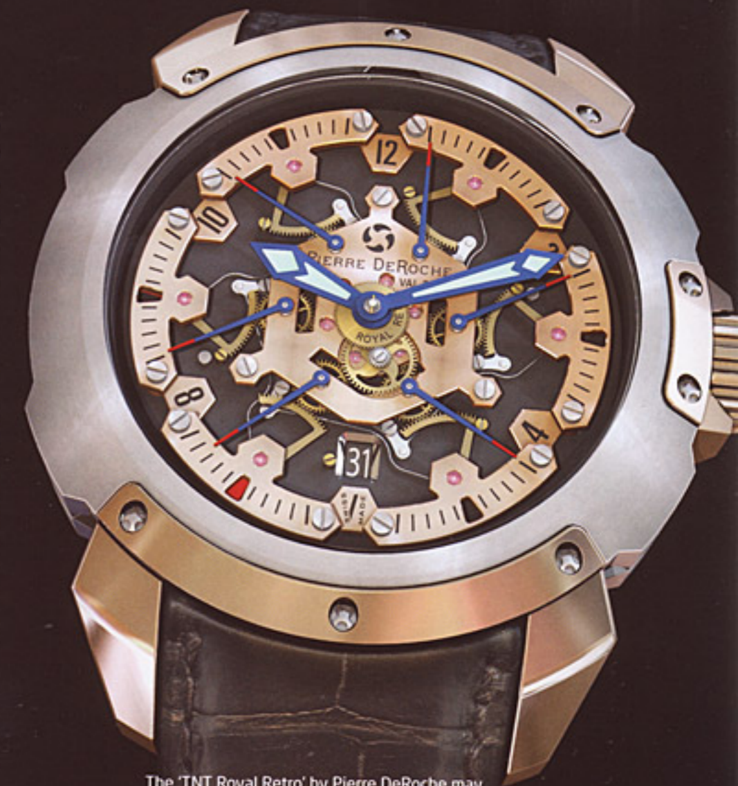
The 'TNT Royal Retro' by Pierre DeRoche may seem a complication too far. It replaces a centre seconds hand with at least 64 additional components. The task of displaying the seconds is split between 6 retrograde hands, the operative hand being indicated by a red flash on the dial. As one hand completes 10 seconds it flicks back and the next one starts; seconds pass around the dial in a relay.
